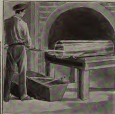
2. The ends of the cylinder are cracked off, and it is cut open with a diamond from end to end. It is then placed in a furnace on a flat surface and the heat causes it to open and flatten out, forming a pane of glass.
